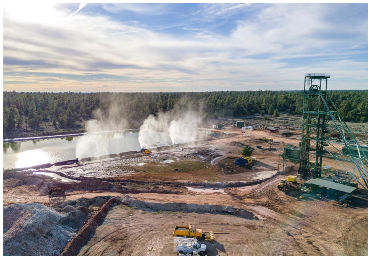
Water cannons spray water pumped from the flooding mine shaft into the air to speed up evaporation.
